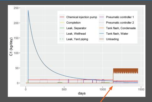
MEET models daily average methane (C1) emissions at a well site from a chemical injection pump, pneumatic controllers, leaks, uncontrolled tank flashes and liquid unloadings over 4 years (1460 days); tank flashes decline over time as production declines; leaks occur and are repaired; pneumatic controllers shift between normal and abnormal emission modes, and unloadings (for gas well liquids) begin after 3 years.
