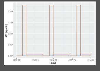
MEET can also model at time scales as short as one second; at day 1,250 of the four-year simulation, gas well liquid unloadings have begun and the site alternates between relatively high emissions due to the unloadings (0.27 kg/min for 60 minutes, three times per day leads to approximately 50 kg/day), much lower emissions when the well is producing but not unloading, and zero emissions when the well is shut in prior to unloading.
